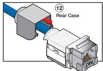
**NOTE:** If there is a need to re-terminate the connector, insert a tweaker on the bottom of the rear case and slide it back to access the wires.
