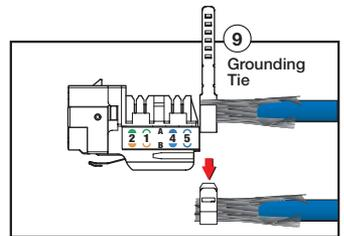
10. Remove the excess braid at the grounding tie.
