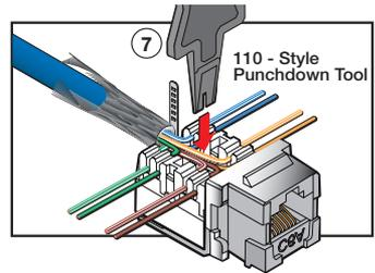
8. Trim the excess wire flush with the body of the connector.
