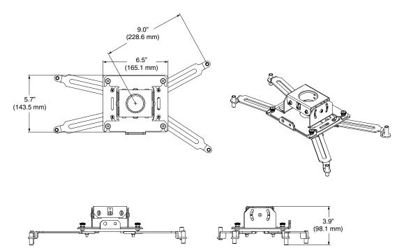
NOTE: The UPB 25 accepts a 1.5" diameter (o.d.), 11.5NPT/NPS pipe.
