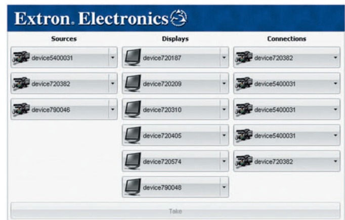
The VN-Matrix Enterprise Controller Switcher utility connects encoder inputs to decoders.
