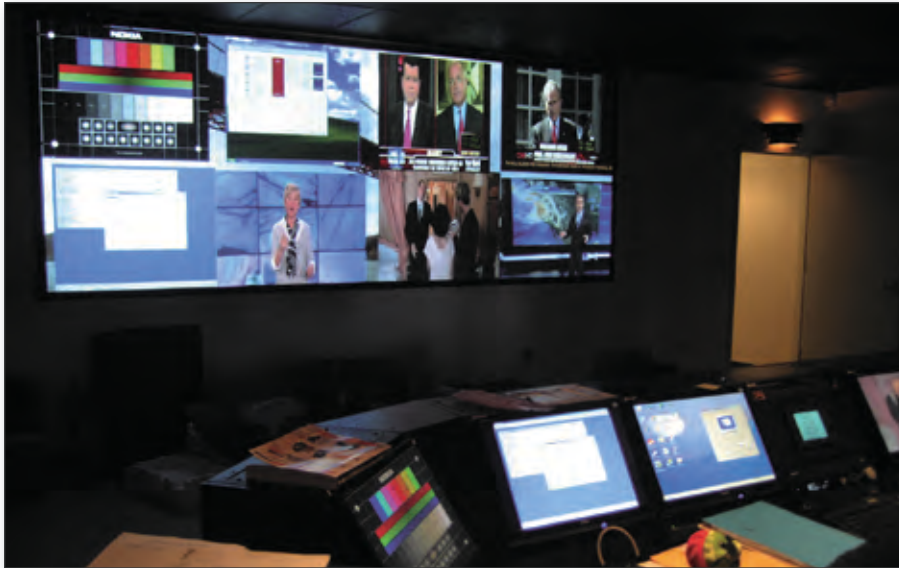
Each window of the WindoWall can show video, HDTV, or high resolution computer-video content.
