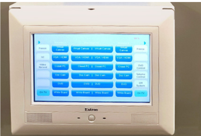
The instructor uses the Extron TLP Pro 720M 7" Wall Mount TouchLink Pro Touchpanel to easily control the system, including setting image windowing and activating streaming/lecture capture.
