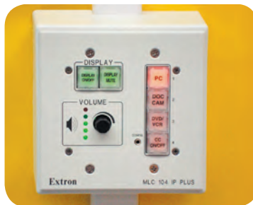
PoleVault System controllers are network connected for remote support and management.
