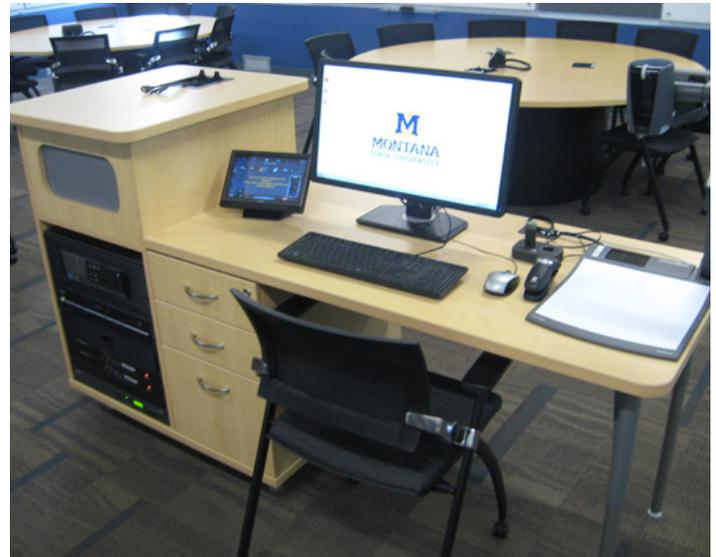
The Extron TLP 1000TV TouchLink Touchpanel enables easy control of the AV system and lighting level to ensure optimal viewing at each table.
