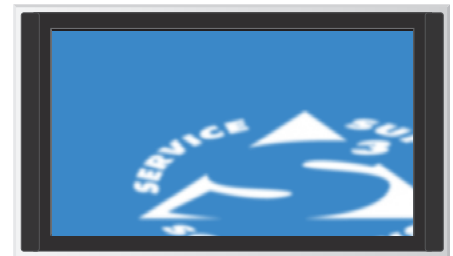
The source resolution does not match that of the display, resulting in a fuzzy, distorted image.
