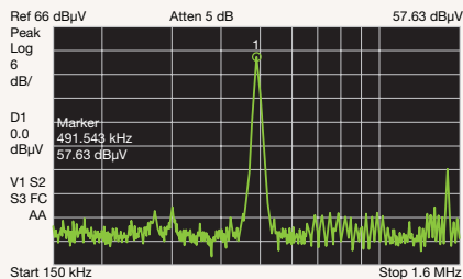
Figure 2 - Fixed Frequency Class D Amplifier Output Cable Emissions
