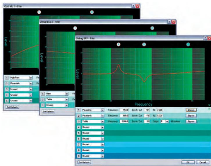
Figure 2: DSP control software can be used to customize and fine-tune DSP filtering functions.
